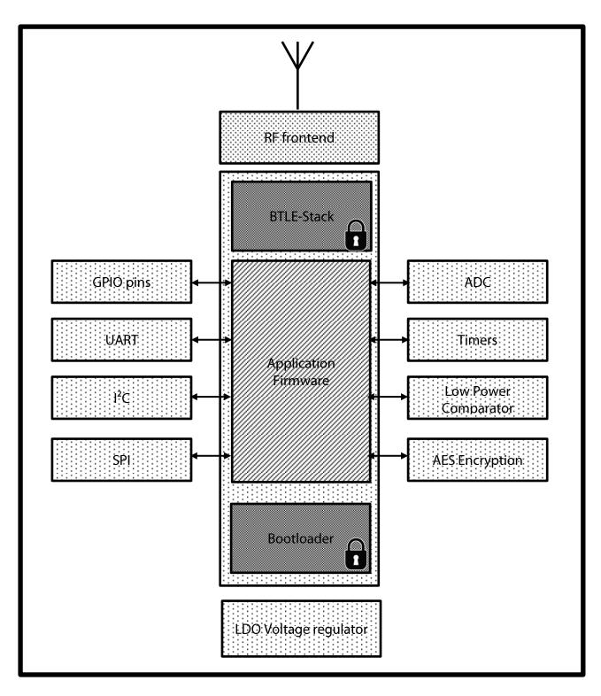
Note: All IO-Interfaces and Data pins are handled by the application firmware only. The BTLE-Stack is shielded from the application firmware to prevent unwanted RF modulation or interference by external data sources.
