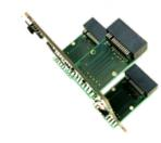
Areus trace adapters enable access to internal control unit interfaces. For instance, debug data can be read out or individual software components can be flashed.
